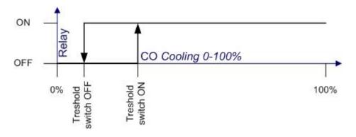
Figure 16: Relay state vs. CO Cooling 0-100%
