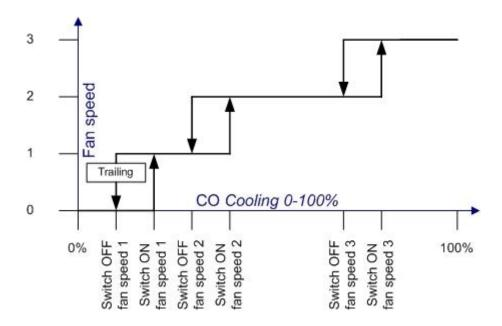
Figure 11: Fan speed vs. CO Cooling 0-100% in automatic mode
