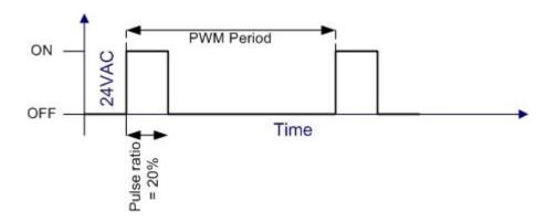
Figure 13: Pulse width modulation: 24VAC vs. time
