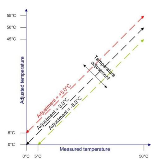
Figure 8b: Adjusted temperature vs. measured temperature
