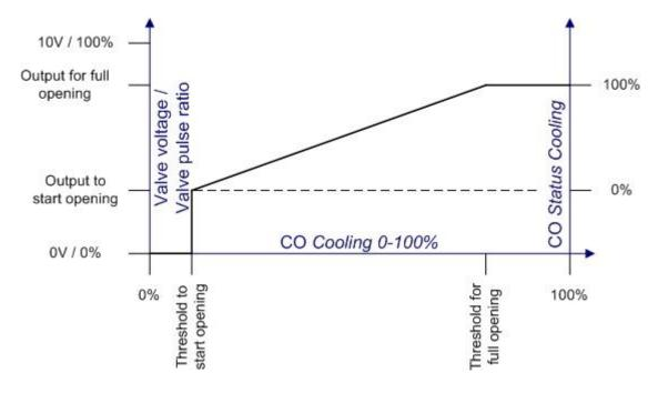
Figure 14: Valve output vs. CO Cooling 0-100%, CO Status Cooling vs. valve output
