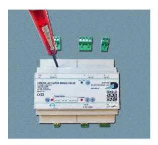
Remove the terminal cover with a screwdriver
