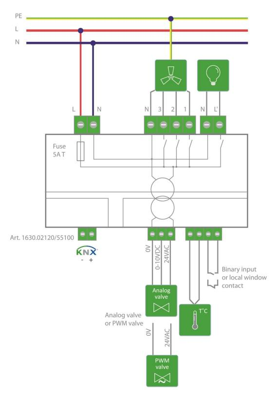
Figure 1: Connection diagram
