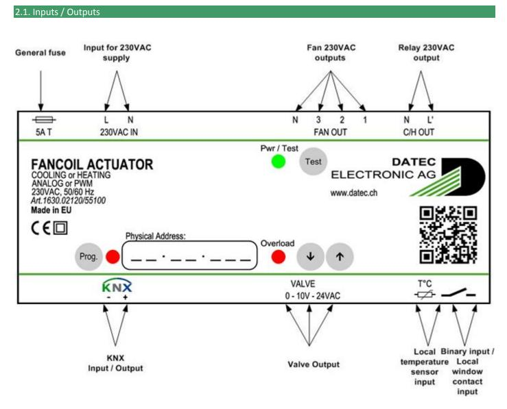
Figure 2: Inputs / Outputs
