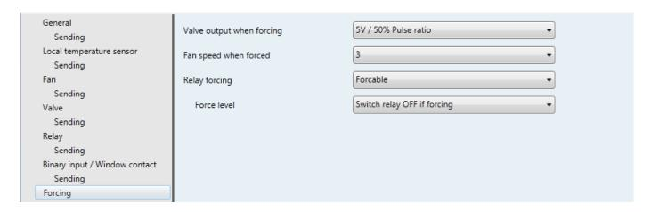
Figure 18: Forcing mode parameters
