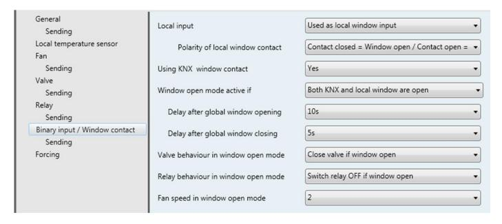
Figure 17: Binary input / Window contact parameters
